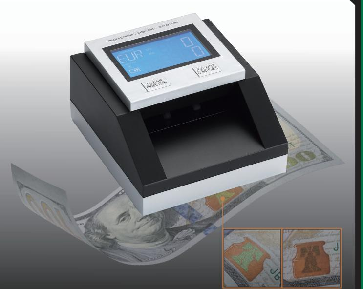
We are ready for detecting USD/EUR/GBP/BDT currencies. Successfully tested in ECB, 100% counterfeit can detected. Detection speed <0.5 sec/note. Upto 6 different Currencies.
